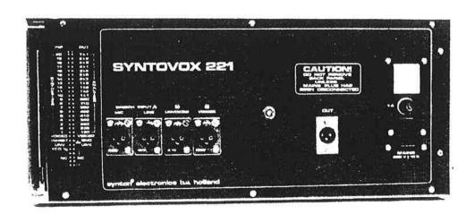
back panel with inputs and output XLRs; mains connector, fuse and mains switch;
