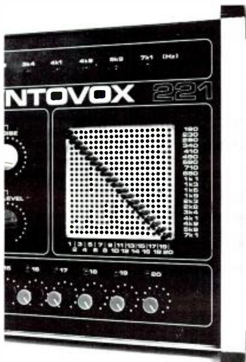
Figure 7. A 20-x-20 matrix connects the analyzer and synthesizer sections of the vocoder.
